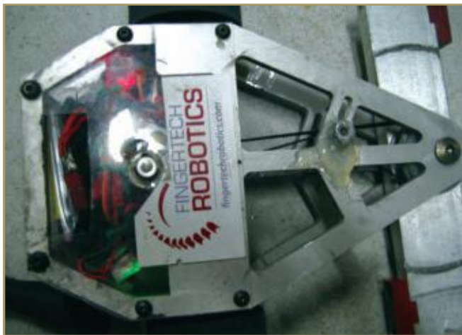
PHOTO 2. Though the robot is a bit bigger than where TinyESCs are usually used, I needed the weight, and the new TinyESCs delivered; they didn't show a hiccup even when running the hot wound B-series motors in a three pound robot!
